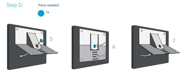
5 Place the blue round foam sticker in the hole of the laptop stand with protection layer removed6 Press down the laptop stand, making sure that the sticker stays properly on the bottom of the laptop7 You can open the laptop stand again. It is now ready for use!
